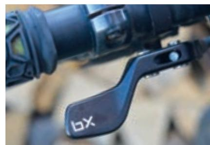
(27.2mm only) in 85 and 105mm drops with a drop-bar lever. The 31.6, 120mm Ascend post I tried weighs about 640g, including lever and cable. It's a penalty of 300-400g over a rigid post but one that's worth paying. If it came to a choice between a suspension fork and a dropper, I'd pick the dropper.
