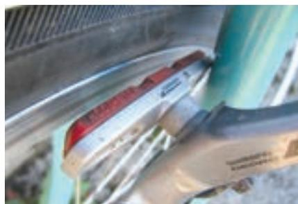
'Salmon' pink compound? Arguably the best known of Kool-Stop's products, it is an 'aggressive' mix formulated for the wet but still, says the maker, superb in the dry. I tested it here as a replacement for Shimano's Deore XT trekking V-brake pads. First up, it works much as claimed; in this installation, in very wet conditions, it is progressive, sensitive, and powerful after a slight delay of perhaps ½ second.
