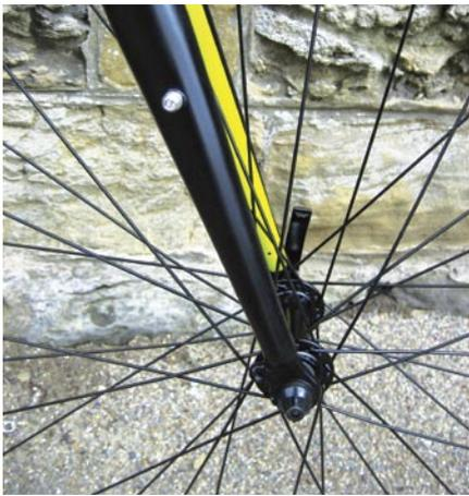
● (Above) The Courier Race has fittings for racks front and rear, in addition to mudguards
